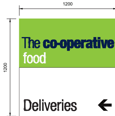
SIGN B Wall mounted Flat Panel with applied vinyl display and anti-graffiti lacquered Non illuminated SCALE 1:20
